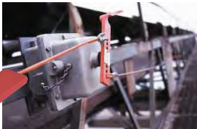
The model RS Safety Stop Switch in operation for immediate shutdown of conveyor system at a sand and gravel company.
