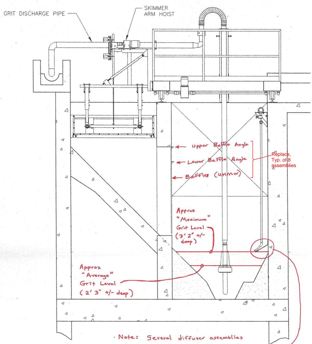
are completely covered with grit. All diffuser assemblies have heavy rag SECTION C-C accumulations.
